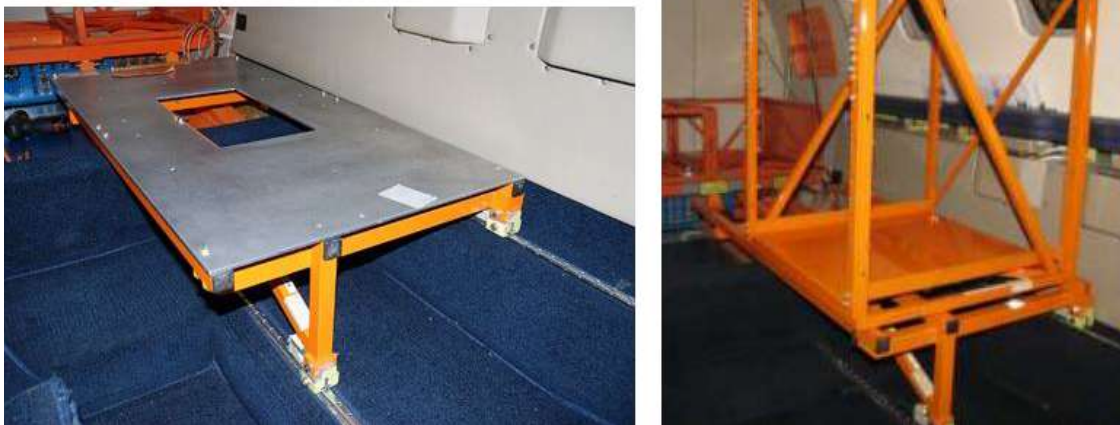
Figure 4: Large cabin platform (left) with 19'' rack installed (right)
