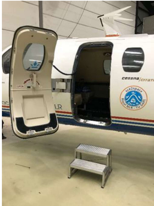
Figure 5: Access Door Dimensions: 1.30 x 0.61 m
