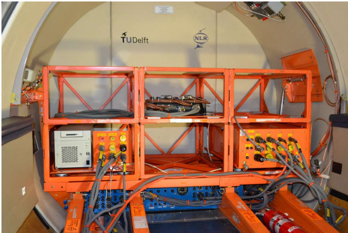
Figure 6: Setup rack in the rear of the Cessna Citation II
