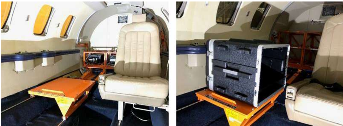
Figure 3: Small cabin platform (left) with empty and unlashed 19'' flight case (right)
